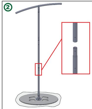
Connect the pipe of holder, then put it into the base
